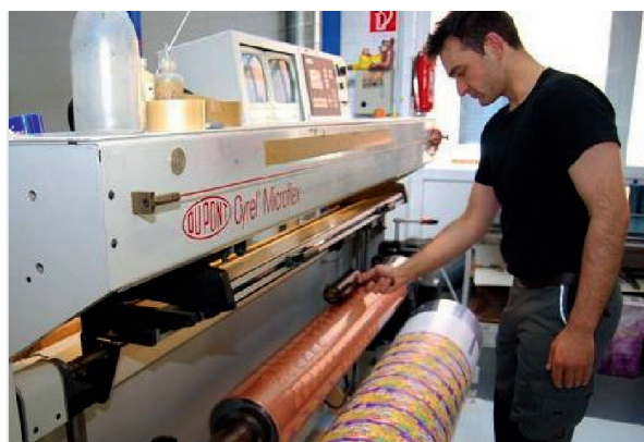
Final "test run" at manufacturer: Individual printing plates were combined to form complete print forms on this round assembly machine and proofing press
