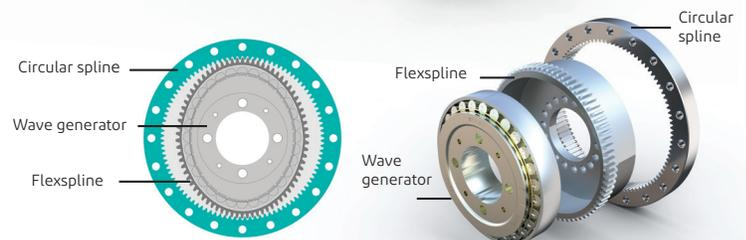
The strain-wave gear set provides repeatable accuracy for positioning inertial loads with high torque. It consists of a circular spline ring gear, a flexspline cup and an elliptical-shaped wave generator that is slightly smaller than the flexible ring and has two fewer teeth. The flexspline deforms to the shape of the wave generator and works independent of the shaft. The flexspline rotates much slower than the wave generator and in the opposite direction.
