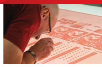
DuPont<sup>™</sup> Cyrel<sup>®</sup> NOWS is an analog medium-high durometer printing plate for high quality process and combination printing. Cyrel<sup>®</sup> NOWS uses proprietary new surface technology to achieve the lowest dot gain, with high ink transfer for smoother solids while retaining all the positive attributes of NOWS.
